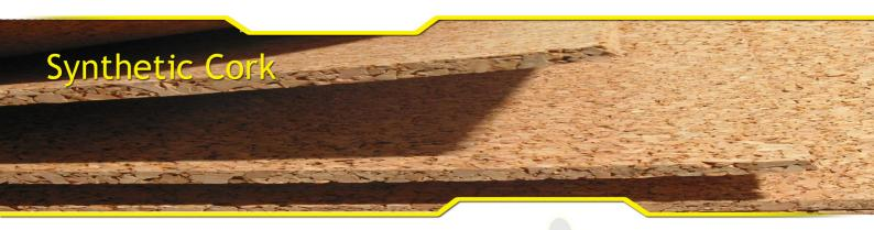
Synthetic Cork is economical, with good oil sealing properties, and resistance to environmental deterioration. Widely used in natural gas meters.
